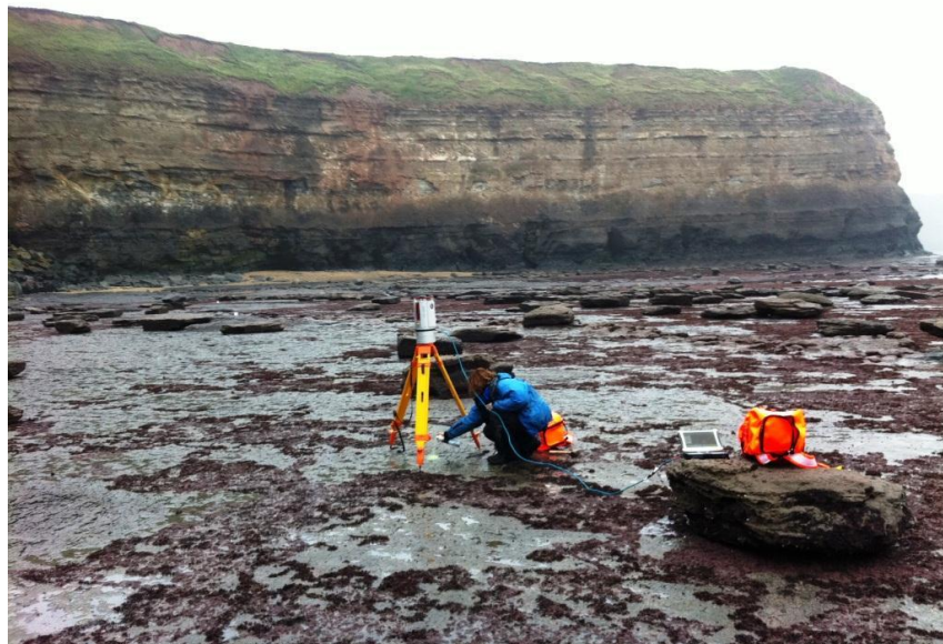
Figure 8 Reigl VZ-1000 at QP1 on the foreshore below Cowbar Nab.
