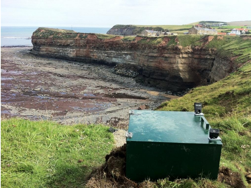
Figure 11 Foreground: Permanent laser scanner installation, showing the view of Cowbar from the scanner housing in the background.
